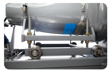
2 Safe handling with lifting equipment and service cart/sled. Horizontal installed Flygt pumps can be equipped with a service cart/sled that ensures safe pump handling.
