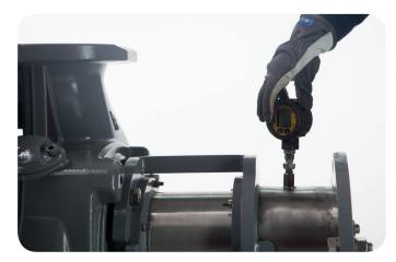
**3** Enhanced performance and efficiency. Horizontally installed pumps benefit from higher available NPSH (Net Positive Suction Head) and no need for shaft alignment compared to vertically installed systems. Additionally, we have added a connection valve for a pressure gauge.
